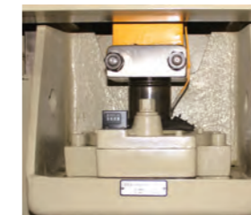
➡ 簡易滑塊調整裝置 (LGN-25) Simple slide adjustment device
